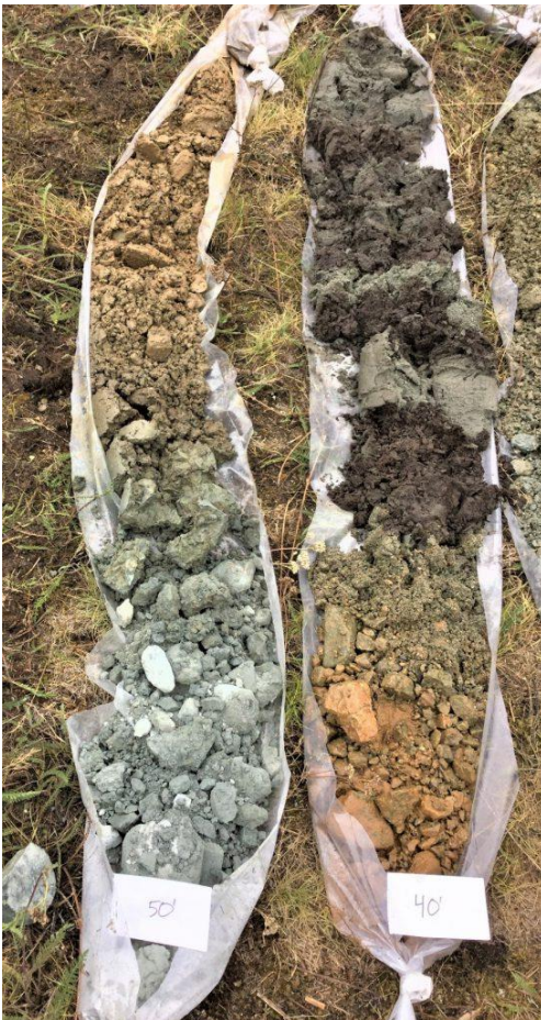
Figure 2: The soil cores in the photo above come from the drilling of Observation Well #478 in Whistler. The core on the left is from 40-50 feet below surface, while the core on the right is from 30-40 feet below surface. The stratigraphy illustrates the changing environment of the area from forested, to wetlands to glacial deposits. Photo credit: Bryan Jackson.
